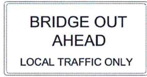
R11 BRIDGE OUT SIGN
