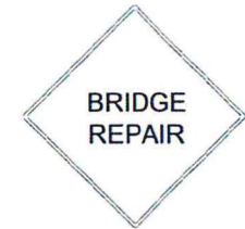
W21-9 BRIDGE REPAIR SIGN
